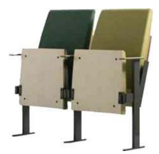
Soft Cushion:High density foam upholstered with durable fabric Seat|Back:Well finished plywood outer back and seat pan Frame:Heavy duty iron frame in powder coated finish Armrest:Quality lacquered nature solid wood Tip-Up Seat:Maintenance free counter weight mechanism Feet:Floor mounting type with 2 bolting holes
